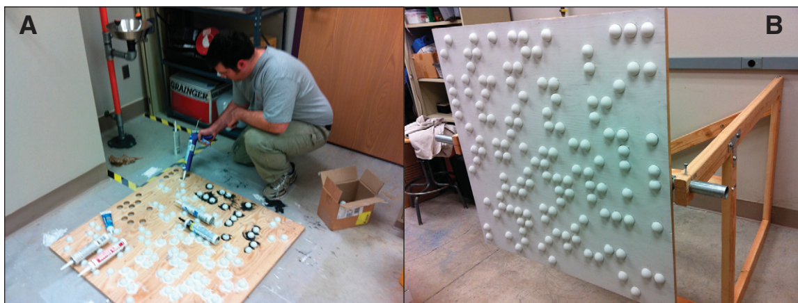
Figure 1. The experimental surface used for this research. (A) Digital image of author fixing roughness elements to the surface using adhesive caulk. (B) Digital image of the completed surface and timber frame.
